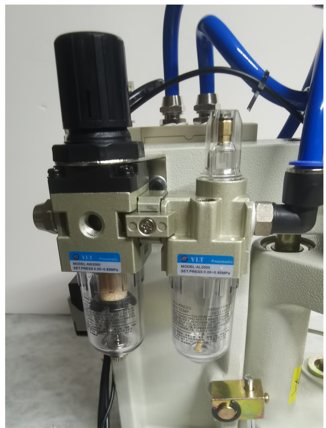
AW2000 Compressed valve and filter
